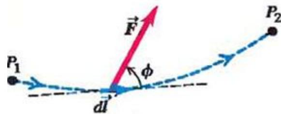
$$W = \int_{P_1}^{P_2} \vec{F} \cos \phi \, d\vec{l} = \int_{P_1}^{P_2} F_{\parallel} \, d\vec{l} = \int_{P_1}^{P_2} \vec{F} \cdot d\vec{l}$$
